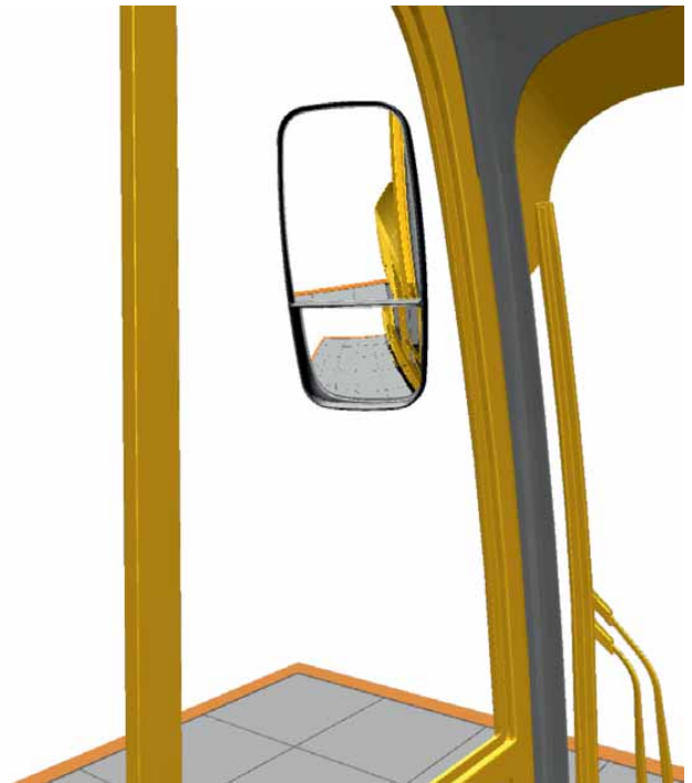
A 3d simulation shows how Ashtree twin lens mirrors can be used to give visibility of areas where there would otherwise be a blind spot
